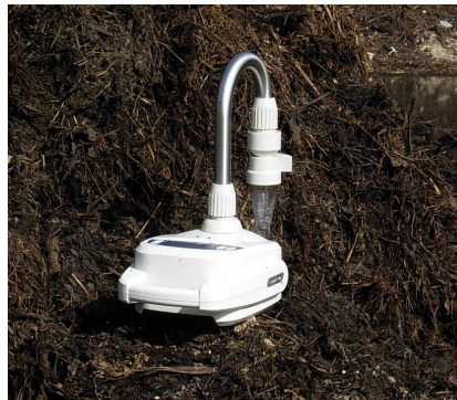
Fig.3 Air sampler "il cigno" at work over a compost heap
